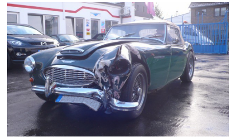
The rear-end collision caused significant damage to the front left-hand side of the Austin-Healey 100-6 BN4.
